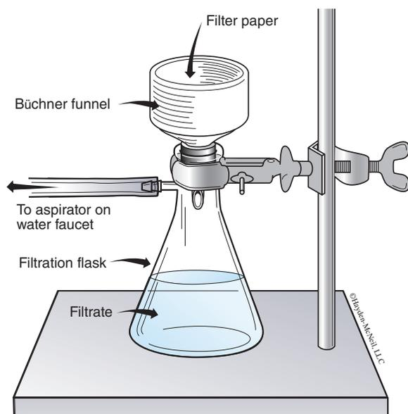
Figure 4.3. Separation technique: Suction filtration.
